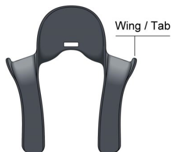
Figure 4 HANS® device model with small tabs on the side of the upper surface of the yokes
