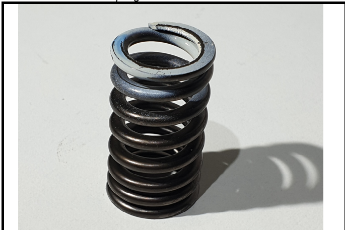
C10-8) Ressort soupape admission Intake valve spring
