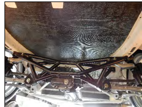
CS4 additional structure external
